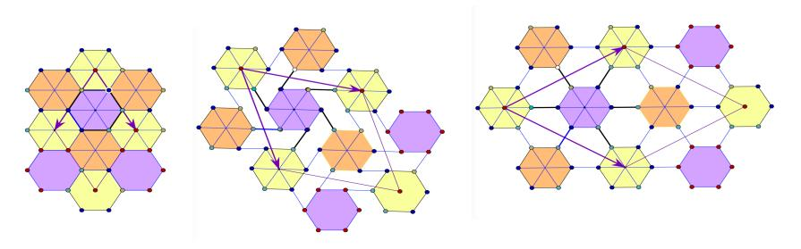
The framework with hexagons has a single degree of freedom and a unique deformation trajectory.
