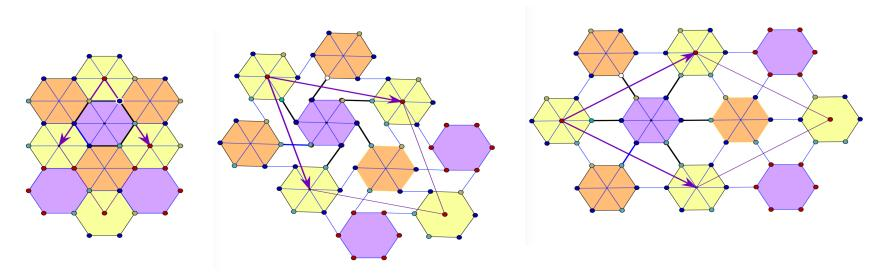
This deployment deformation is auxetic since the Gram map goes to increasing scalar multiples of the Gram matrix for the tiling.
