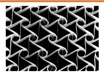
From D. Prall and R.S. Lakes: PROPERTIES OF A CHIRAL HONEYCOMB WITH A POISSON'S RATIO OF - 1 *Int. J. Mech. Sci.* Vol. 39, No. 3, pp. 305 314. 1997
