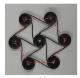
Hexachiral version from F. Scarpa et al. **Shape memory polymer hexachiral auxetic structures with tunable stiffness,** Smart Mater. Struct. **23** (2014) 045007
