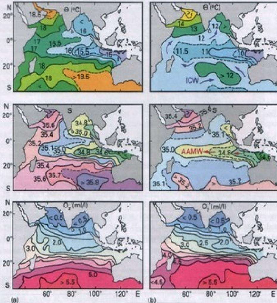
Fig. 12.9. Annual mean temperature ( $^{\circ}\text{C}$ ), salinity, and oxygen (ml/l) in the thermocline on isopycnal surfaces. (a) On the  $\sigma_{\theta}$  surface 25.7, located in the depth range 150 - 200 m, (b) on the  $\sigma_{\theta}$  surface 26.7, located in the depth range 300 - 450 m. Arrows indicate the movement of ICW and AAMW. After You and Tomczak (1993)
