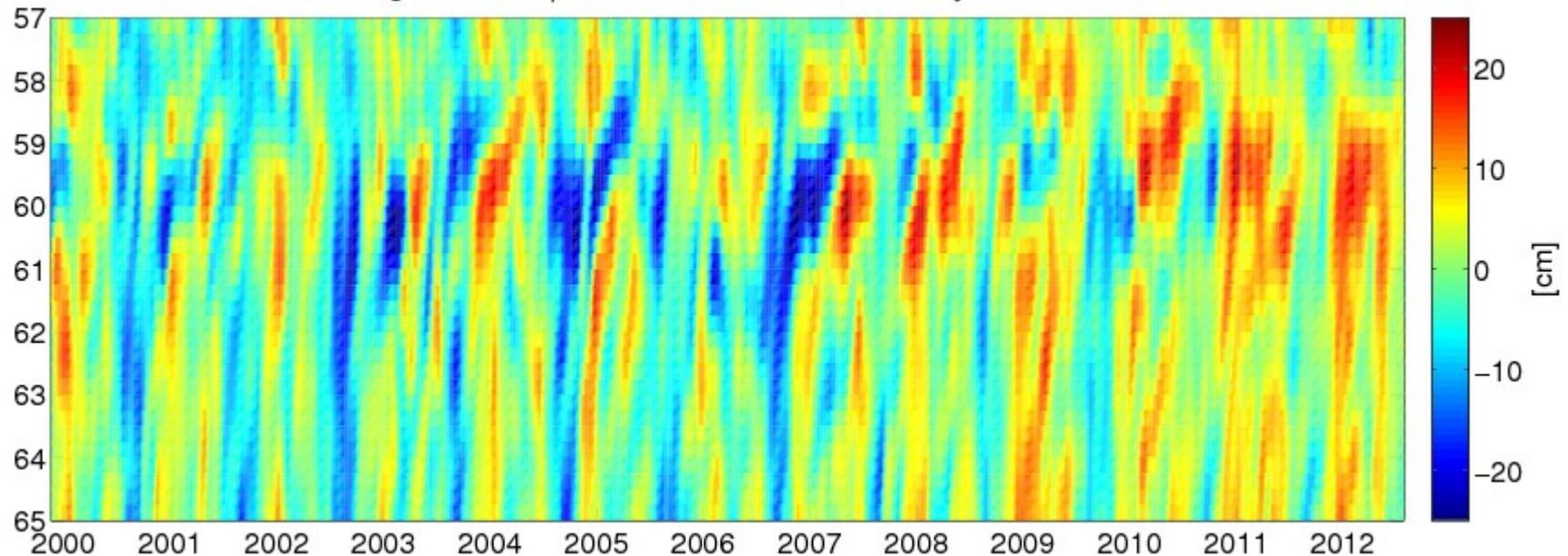
A Rossby Wave with wavelength  $\sim 500$  km and phase speed 2.5 cm/s propagates along 24.30N and brings positive SSH near 60E at the end of winter. This SSH is intensified there
