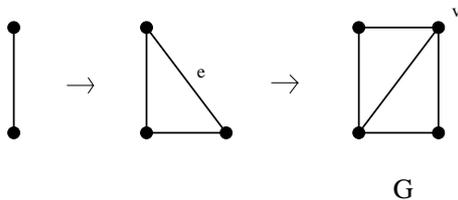
FIGURE 1. A recursive construction of a  $(2, 3)$ -tight graph  $G$  from the complete graph on two vertices,  $K_2$ , by applying a Henneberg 1 move and then a Henneberg 2 move.
