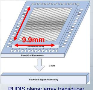
PUDIS planar array transducer design with 32x32 elements
