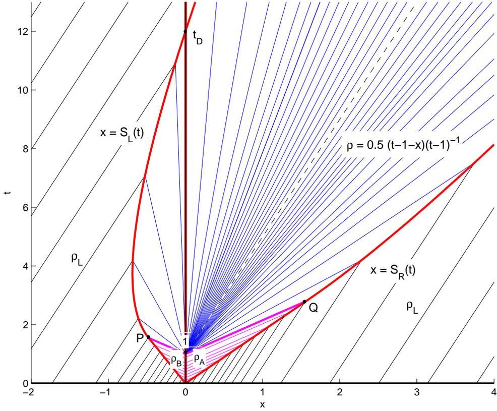
**Figure 4:** *Light traffic.* The characteristic projections and shock curves on the  $(x, t)$  plane for  $\rho_L = 3/8$  and  $\lambda = 1/2$ . The left shock curve crosses the point  $x = 0$  at  $t_D = 12$ . The dotted line starting at  $(0, 1)$  is the dividing characteristic (54).
