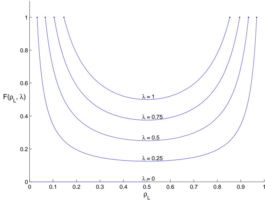
**Figure 2:** Ratio  $F(\rho_L, \lambda)$  of the traffic flux out of the road block to the traffic flux into the left shock plotted against the traffic density on the open road  $\rho_L$  for  $\rho_A \leq \rho_L \leq \rho_B$  and for a range of values of  $\lambda$ .
