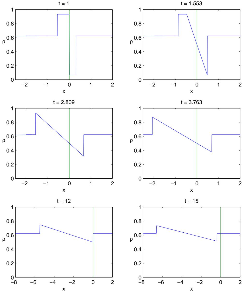
**Figure 11:** Heavy traffic. Traffic density plotted against  $x$  for  $\rho_L = 5/8$ ,  $\lambda = 1/2$  and  $t = 1$ ,  $t = t_Q = 1.553$ ,  $t = t_P = 2.809$ ,  $t = 3.763$ .  $t = t_D = 12$  and  $t = 15$ . At time  $t = 3.763$  the shock has reached its maximum distance behind the road block.
