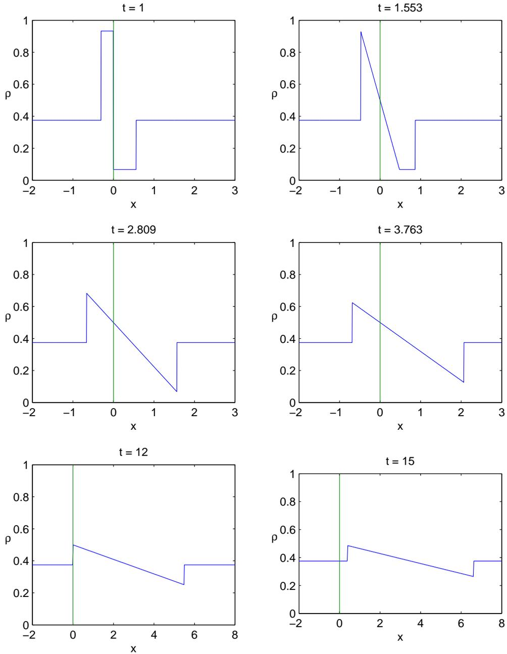
**Figure 7:** *Light traffic. Traffic density plotted against  $x$  for  $\rho_L = 3/8$ ,  $\lambda = 1/2$  and  $t = 1$ ,  $t = t_P = 1.553$ ,  $t = t_Q = 2.809$ ,  $t = 3.763$ ,  $t = t_D = 12$  and  $t = 15$ . The length of the tailback is maximum at  $t = 3.763$ .*
