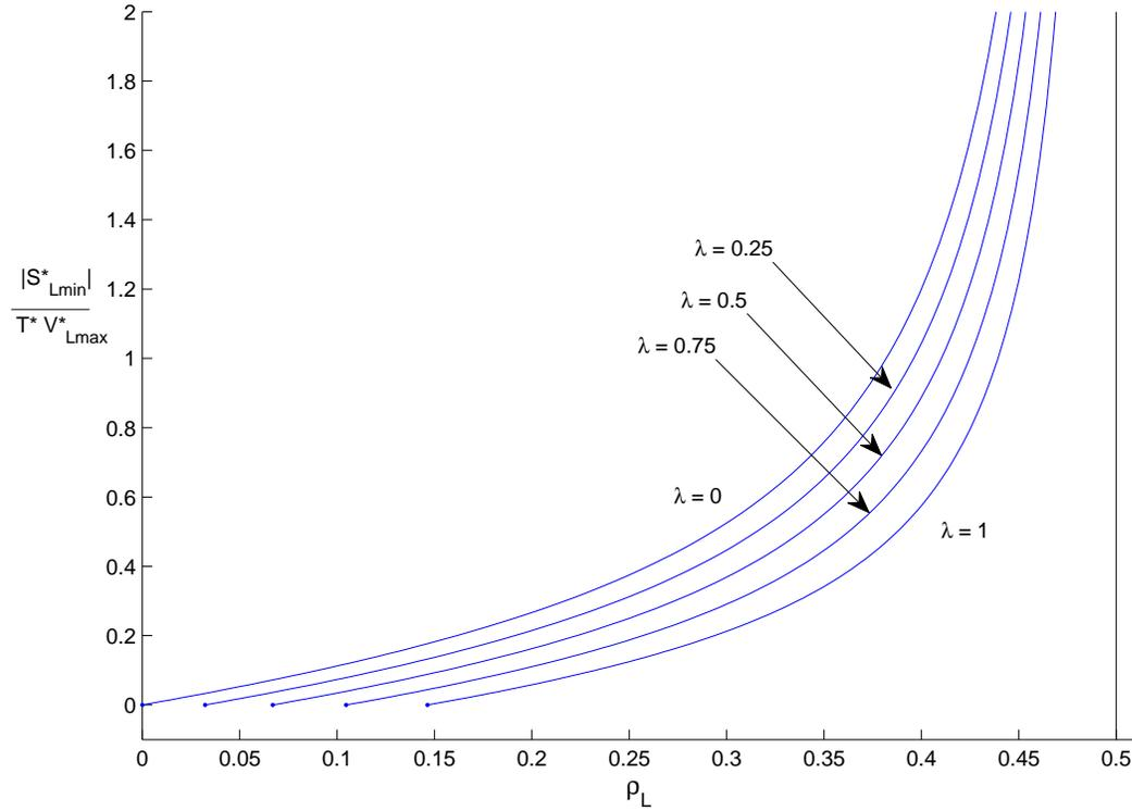
**Figure 5:** Road block removed. Maximum length of the tailback, scaled by  $T^* V_{L\max}^*$ , plotted against the traffic density on the open road  $\rho_A \leq \rho_L < 1/2$  and for a range of values of  $\lambda$ .
