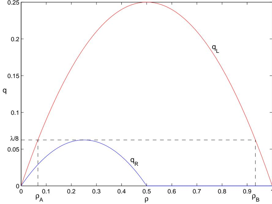
**Figure 1:** The traffic flux in the open road,  $q_L$ , and in the road block,  $q_R$ , plotted against the traffic density  $\rho$  for  $\lambda = 1/2$ . The traffic densities  $\rho_A$  and  $\rho_B$  are defined by (10) and (11).
