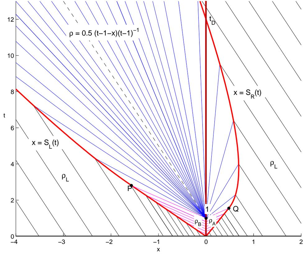
**Figure 10:** *Heavy traffic. The characteristic projections and shock curves on the  $(x, t)$  plane for  $\rho_L = 5/8$  and  $\lambda = 1/2$ . The right shock curve crosses the point  $x = 0$  at  $t_D = 12$ . The dividing characteristic (54) has negative gradient and is the dotted line starting at  $(0, 1)$ .*
