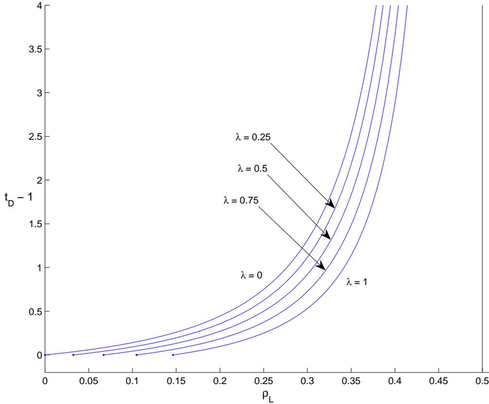
**Figure 6:** Ratio of the additional time taken for the effects of the road block to clear to the time the road block was in place,  $t_D - 1$ , plotted against  $\rho_L$  for  $\rho_A \leq \rho_L < 1/2$  and for a range of values of  $\lambda$ .
