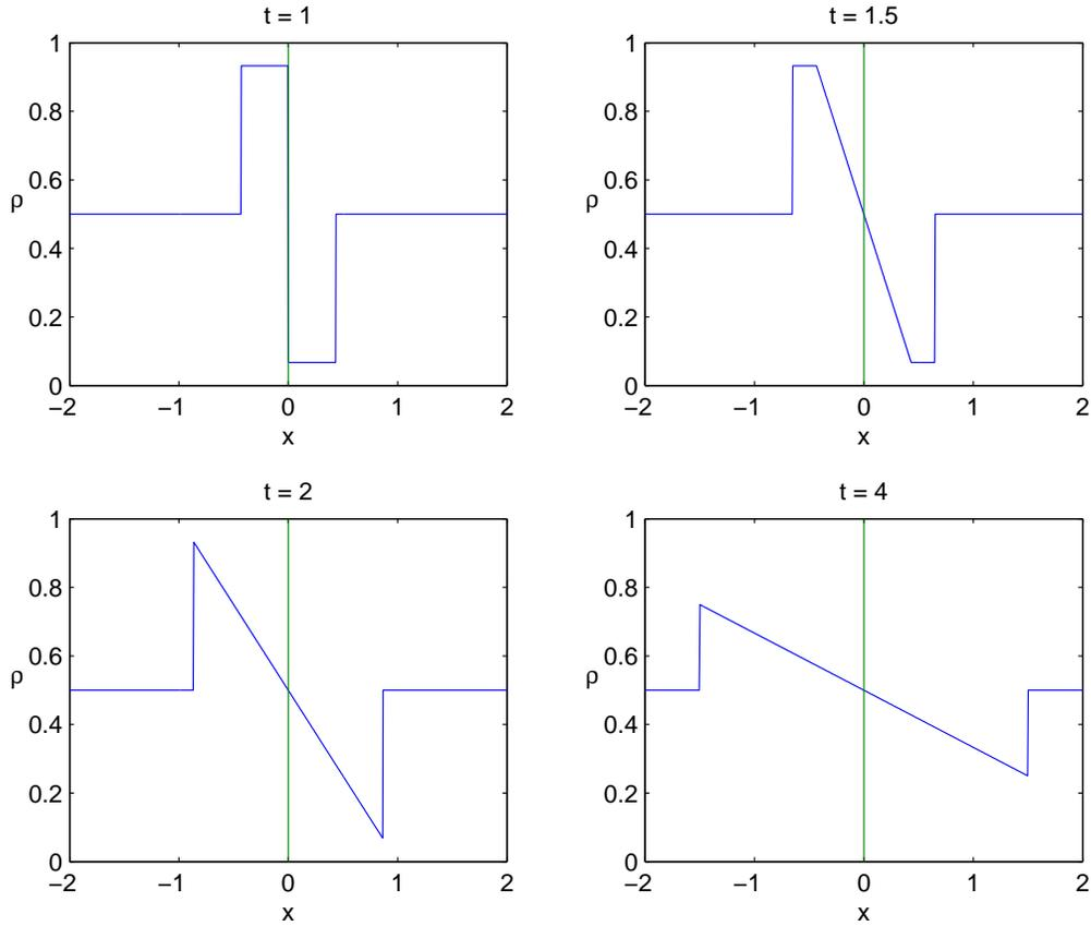
**Figure 9:** *Critical traffic flux. Traffic density plotted against  $x$  for  $\rho_L = 1/2$ ,  $\lambda = 1/2$  and  $t = 1$ ,  $t = 1.5$ ,  $t = t_P = t_Q = 2$  and  $t = 4$ .*
