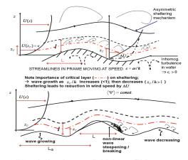
Note growing/decreasing wave amplitude in the group. This increases critical height  $z_c$  (---) on downwind side of group  $-cch_0$  where wave shape changes
