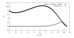
Figure: Component of energy transfer parameter,  $\beta_c$ , due to inertial critical layer for growing waves (where  $c_i \ll U_*$ ) as a function of the wave age  $c_r/U_1$ . •, numerical solution of inviscid Orr-Sommerfeld equation for  $c_i = 0$  and  $\nu_e = 0$  using the singular critical layer approach;  $\circ$  numerical solution of equation IN-Rayleigh equation for  $c_i \neq 0$  and  $\nu_e \neq 0$ .
