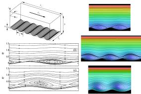
Flow over moving waves is attached to the mean flow.
