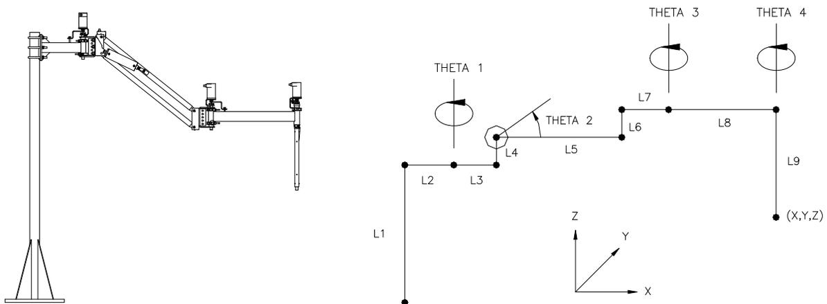
Figure 1. Measurement arm
