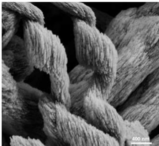
**Figure 20.** SEM image of helical  $\text{BaCO}_3$  fibers formed in presence of a stiff phosphonated block copolymer. Reproduced from ref. [84] with permission of Nature Publishing Group.
