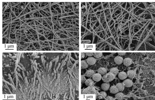
**Figure 2.** SEM images of  $\text{BaCO}_3$  crystals after 1 day of growth at starting pH values of a) 1.8, b) 3.5, c) 5.5, and d) 6.5 ([polymer] =  $1\text{ g L}^{-1}$ ,  $[\text{Ba}^{2+}] = 10\text{ mM}$ ).
