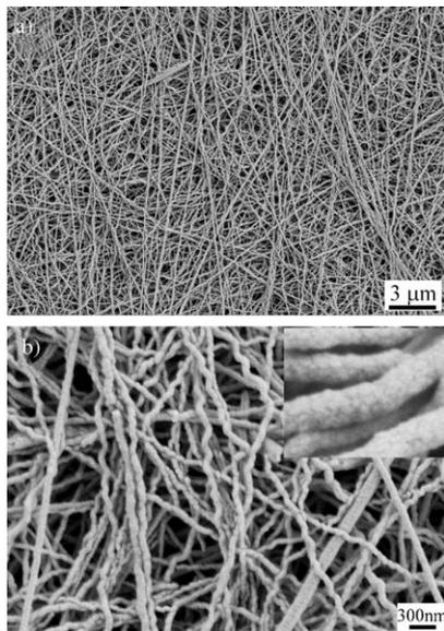
**Figure 1.** SEM images at different resolutions of ultralong nanofibers of  $\text{BaCO}_3$  after 1 day of growth ([polymer] =  $0.5\text{ g L}^{-1}$ ,  $[\text{Ba}^{2+}] = 20\text{ mM}$ , starting pH 3.5); inset in (b) is an enlargement.
