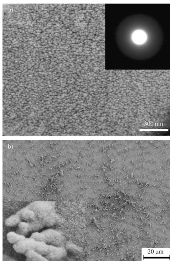
**Figure 4.** SEM images of the BaCO<sub>3</sub> particles after a) 4 h and b) 18 h of growth ([polymer]=1 g L<sup>-1</sup>, [Ba<sup>2+</sup>]=10 mM, starting pH 5.5); inset in (a) is the corresponding ED pattern; inset in (b) is an enlargement.
