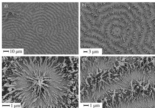
**Figure 3.** SEM images at different resolutions of the concentric ring patterns of BaCO<sub>3</sub> crystals after 1 day of growth ([polymer] = 1 g L<sup>-1</sup>, [Ba<sup>2+</sup>] = 10 mM, starting pH 5.5).
