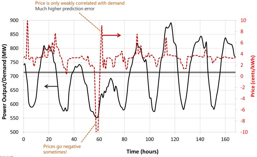
**Source:** Nease J, Adams TA II. Rolling-Horizon Optimization of Integrated Solid-Oxide Fuel Cell and Compressed Air Energy Storage Plant for Zero-Emissions Peaking Power. Submitted (2014)
