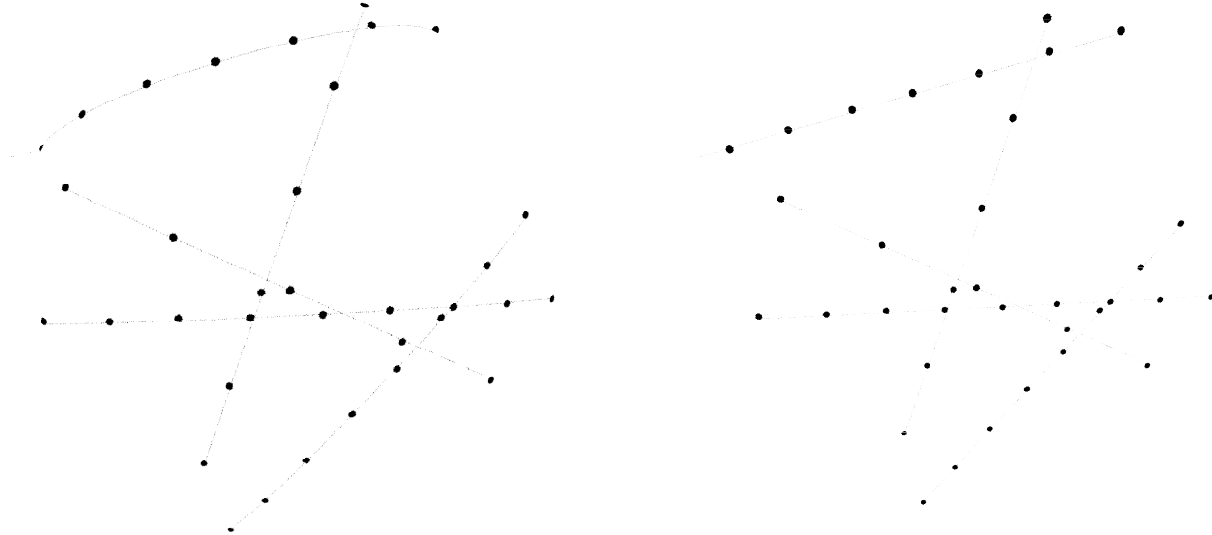
Figure 1: On the left, the observed data is seen in perspective and with a certain amount of distortion, which may include random perturbations modeled as noise. On the right, the original data originates from a set of straight lines. On each straight line, the original points are equally spaced, but this spacing may not be the same from one line to the next. A typical situation has at most 30 lines and between 8 and 25 points on each.
