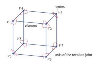
Counting: m-s = -6: no indication of a mechanism
