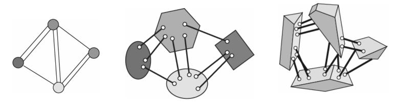
Tay's theorem (Tay 1984). A d-dimensional body-bar framework (G, b) is rigid for a "generic" bar-configuration b iff G contains  $\binom{d+1}{2}$  edge-disjoint spanning trees.
