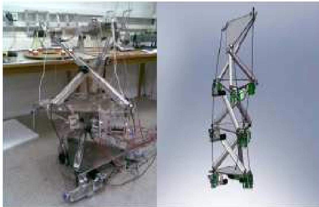
Fig. 4a: The two floor prototype robot (left) and a model of the three floor prototype (right)
