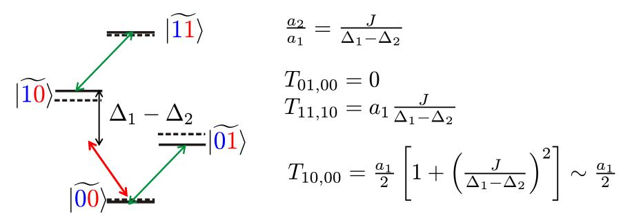
Leakage effects when  $T_{10,00} \sim \Delta_1 - \Delta_2$ Maximum gate speed  $T_{11,10} < J$
