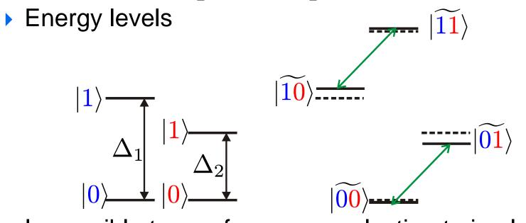
• Impossible to use frequency selection to implement a CNOT gate:  $\omega_{_{10,11}} = \omega_{_{00,01}}$
