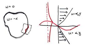
Surface waves propagate along discontinuity, decay exponentially into the interior.
