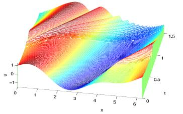
Solution for real part  $u = \Re \psi$  of  $\psi_t = \mathbf{P} \partial_x \left[ \psi |\partial_x| n - n |\partial_x| \psi \right]$
