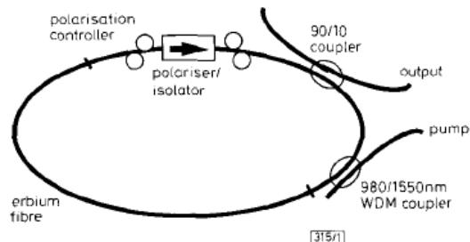
Tamura, Haus, and Ippen, "Self-starting additive pulse mode-locked erbium fiber ring laser," Electron. Lett. **28**, 2226 (1992)
