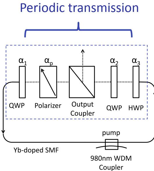
$$Q = \frac{1}{2} \left\{ e^{-iK} [\cos(2\alpha_2 - 2\alpha_3 - \alpha_p) + i \cos(2\alpha_3 - \alpha_p)] \right. \\ \times [i \cos(2\alpha_1 - \alpha_p - w) - \cos(\alpha_p - w)] \\ + e^{iK} [\sin(2\alpha_2 - 2\alpha_3 - \alpha_p) - i \sin(2\alpha_3 - \alpha_p)] \\ \left. \times [\sin(\alpha_p - w) - i \sin(2\alpha_1 - \alpha_p - w)] \right\} .$$
