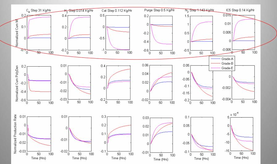
Step responses at three operating points for a polymer process
