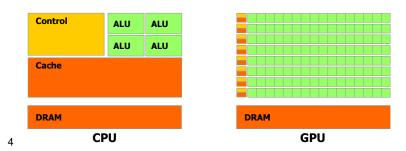
More transistors are dedicated to data processing rather than data caching and control flow. GPUs typically have hundreds of cores. (Tesla C2050 — 448 cores)
