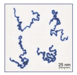
Appearance of real linear polymer chains as recorded using an atomic force microscope on surface under liquid medium. Chain contour length is 204 nm; thickness is 0.4 nm. (Roiter and Minko, 2005).
