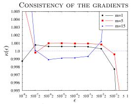
$$\kappa(\epsilon) \triangleq \frac{\mathcal{J}(\phi + \epsilon \phi') - \mathcal{J}(\phi)}{(\nabla \mathcal{J}, \phi')}, \text{ where } \phi'(t) = \sin\left(m2\pi \frac{t}{T}\right)$$
