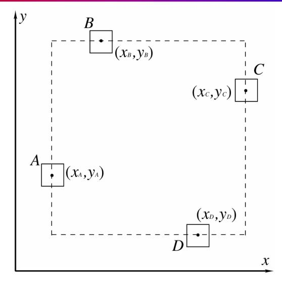
An example of four-module nets with bounding box
