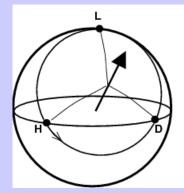
Use fixed waveplates plus one Pockels cell (with *three* voltages: 0, ±V)
