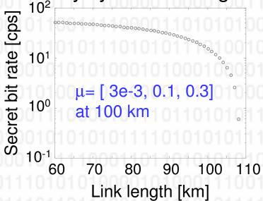
Creation of PNS-secure key over 107 km of optical fiber\*, an increase of 80% over previous highest reported distance of 60 km (see H.-K. Lo quant-ph/0601168)
