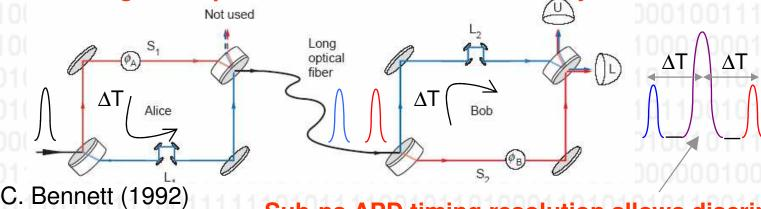
Sub-ns APD timing resolution allows discrimination of central (long-short + short-long) time bin for QKD
