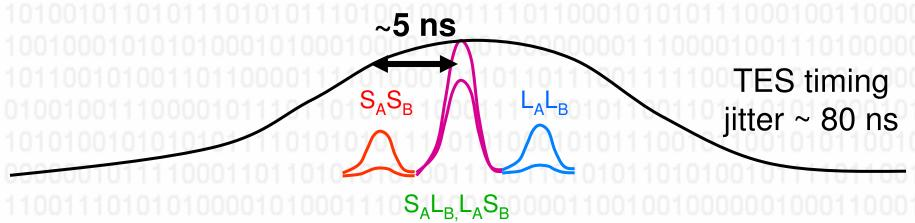
Switch is set to route all  $S_A$  ( $L_A$ ) photons from Alice to  $L_B$  ( $S_B$ )
