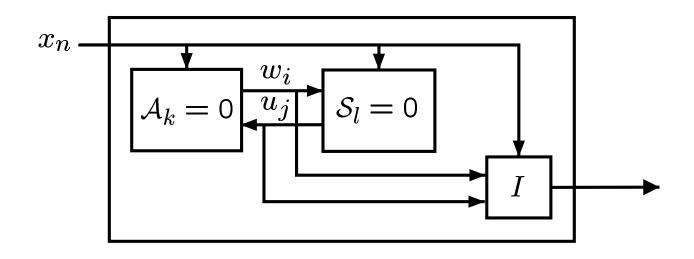
Two coupled disciplines: Aerodynamics  $(A_k)$  and Structures  $(S_l)$ .
