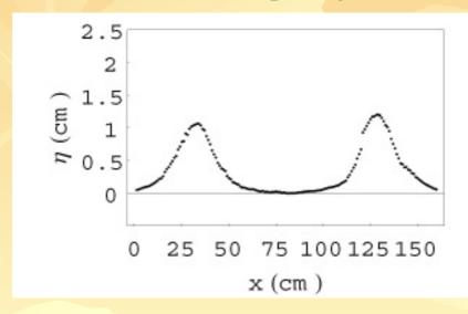
Shift based on the reflected wave passage over the pressure gage.
