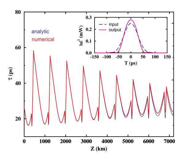
Optimize chirp+transmission to minimize pulse width at receiver Can show analytically that nonlinearity reduced by  $O(\log s/s)$  [26]
