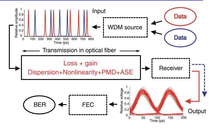
WDM, wavelength-division multiplexing PMD, polarization mode dispersion ASE, amplified spontaneous emission noise FEC, forward error correction BER, bit-error ratio
