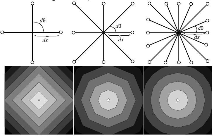
Grids for the 5, 9, and 17 point schemes, and level sets of the cones for the corresponding schemes.
