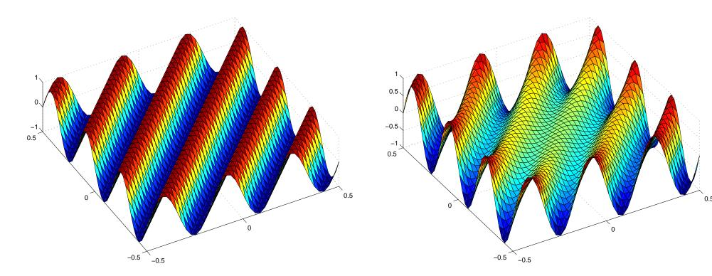
Solution of the centered scheme differs by 1 from the exact solution.
