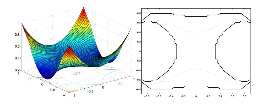
Solution and free boundary for the nonconvex, fully nonlinear second order equation  $\max(\min(L^1u, L^2u)L^3u) - 1$ .
