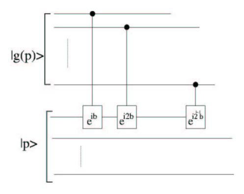
b is the control bit. The circuit uses I controlled 1-qubit phaseshifts.
